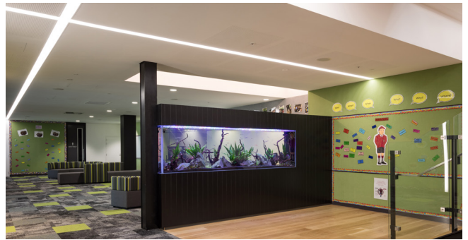
Image 1: Example of 90° mitres in recessed Energyline
