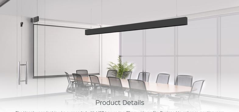
The Heaphy pendant is wire suspended with UGR Louvre in a 75mm wide profile. Designed to enhance meeting room spaces, the multi cell louvre delivers a visually comfortable space for people to enjoy, with square louvre openings achieving excellent cut off angles below 45°.
