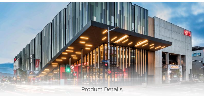
Delivering IP54 protection in a 75mm housing, Milford is ideal for recessing under canopy shop fronts or other wet locations. These products serve a dual purpose - visually great spaces as well as achieving functional lighting in exterior spaces.
